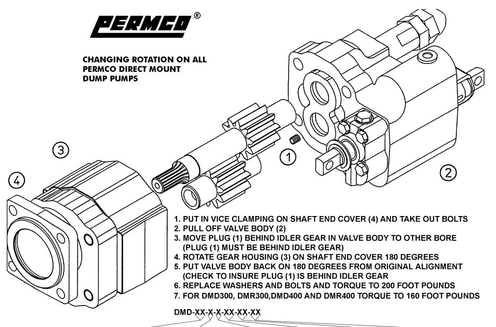
GEAR SIZE X-2 LINE R-RIGHT HAND AS-AIR SHIFT RELIEF VALV (15, 20, 25) Z-3 LINE W/SLEEVE L-LEFT HAND MS-MANUAL SHIFT 20-2000 PSI
